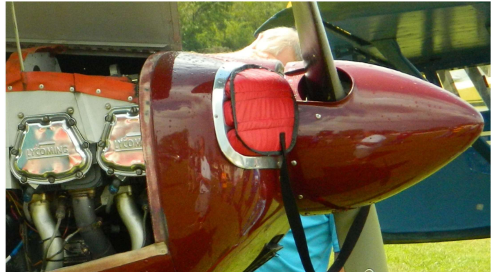
Flat-4 Lycoming O-360 replacing original Franklin engine in a Stinson 108-3 (author)
