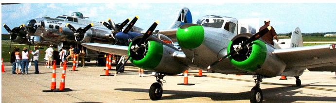
Twin Jacobs radials powered the World War II Cessna Bobcat, which trained American, Canadian and British pilots to fly transports & bombers, including the B-17 Flying Fortress (background) (author)
